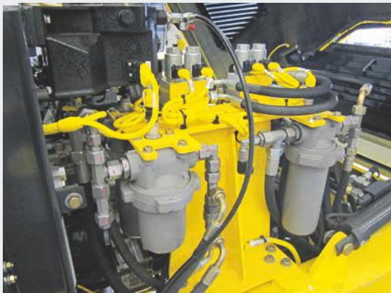
Discharge side of the hydraulic filter system.
