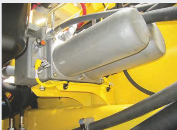
Electronic monitoring of hydraulics return filter system.
