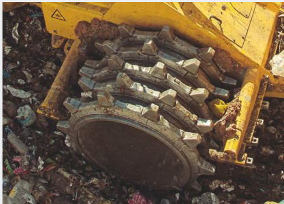
Clean wheels with effective scrapers (optimum compaction).
