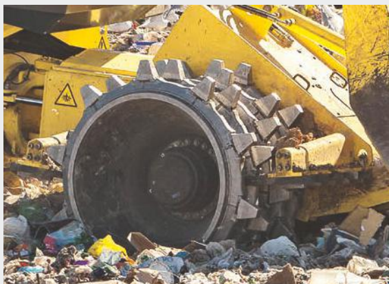
Scrapers guarantee clean wheels and high compaction.
