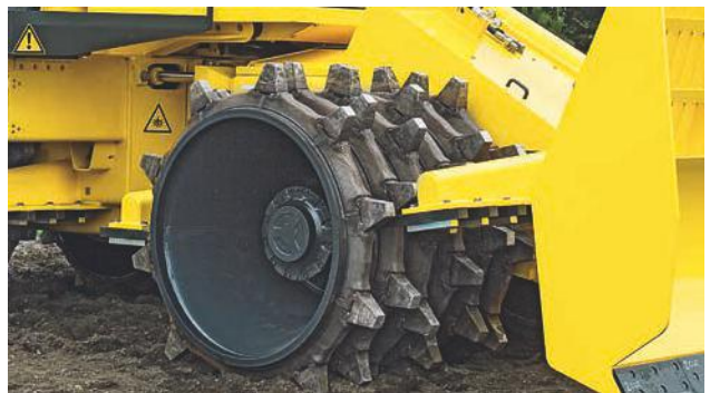
Welded wheel bodies with inner taper on both sides for optimum stability (premium).
