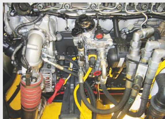
Multi-stage fuel filtering.
